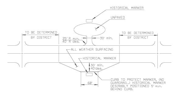
Figure 334-A Example of Geometrics Of a Pull-Out For a Historical Marker Site
