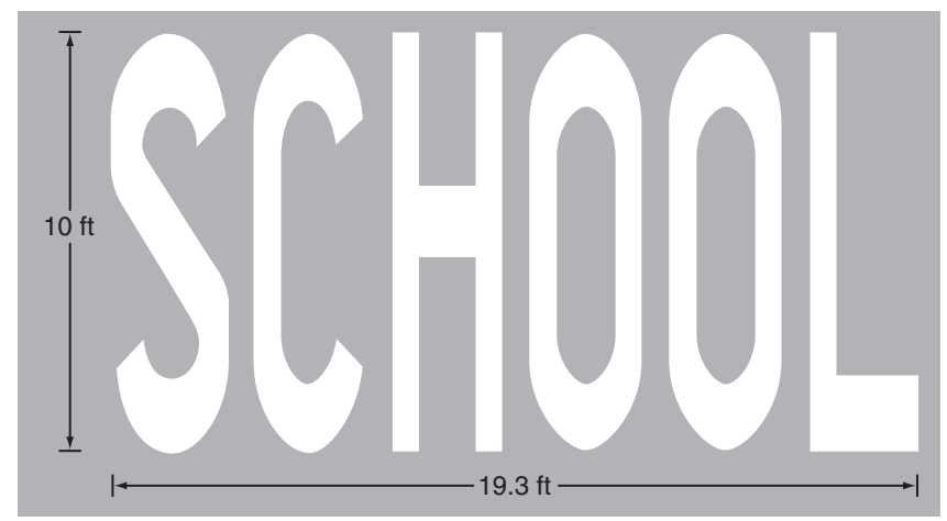
Figure 7C-1. Two-Lane Pavement Marking of "SCHOOL"
