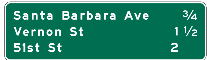
Figure 2E-31. Interchange Sequence Sign
