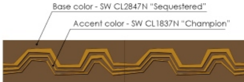
BRIDGE BARRIER WALL PATTERN
