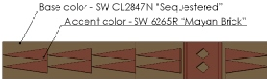
BRIDGE BARRIER WALL PATTERN
