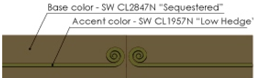
BRIDGE BARRIER WALL PATTERN
