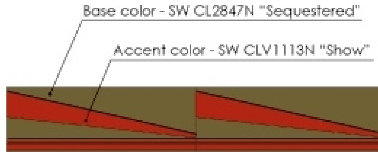
BRIDGE BARRIER WALL PATTERN
