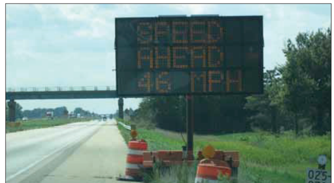
Figure 1. A portable changeable message sign providing downstream traffic speeds from sensor data.
