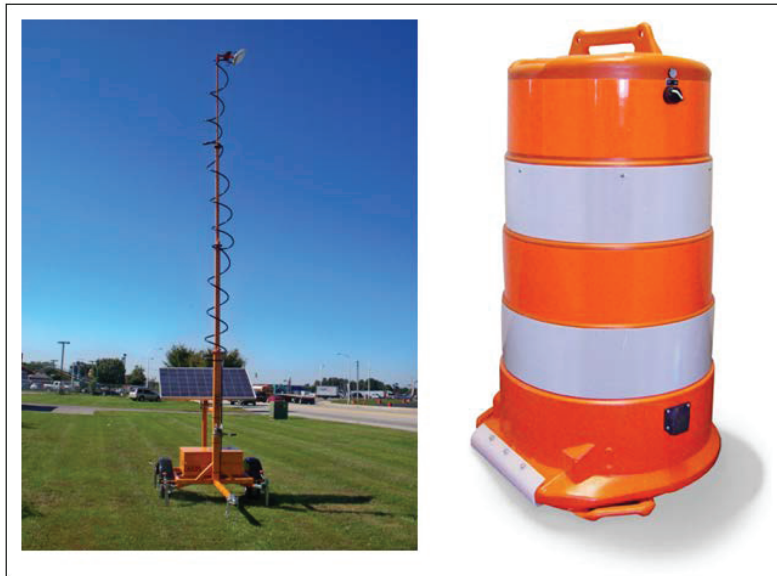
Figure 5: Portable Traffic Sensor (PTS) (microwave) and an iCone® (radar)
