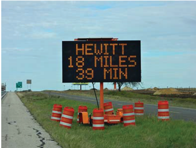
This dynamic message sign provides travelers with real-time information on the expected travel time to the indicated destination.
