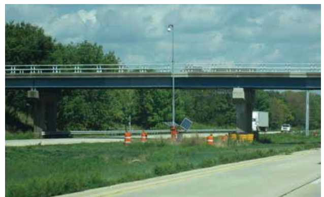
Figure 2. Temporary, solar-powered vehicle detection and camera systems.
