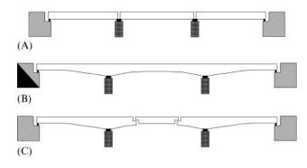
**Cantilever:** Cantilevers are structures that project horizontally into space supported on only one end. Smaller cantilevers are simple beams. Larger ones use trusses made from structural steel or box girders built from concrete. Cantilever bridges can span relatively long distances.
